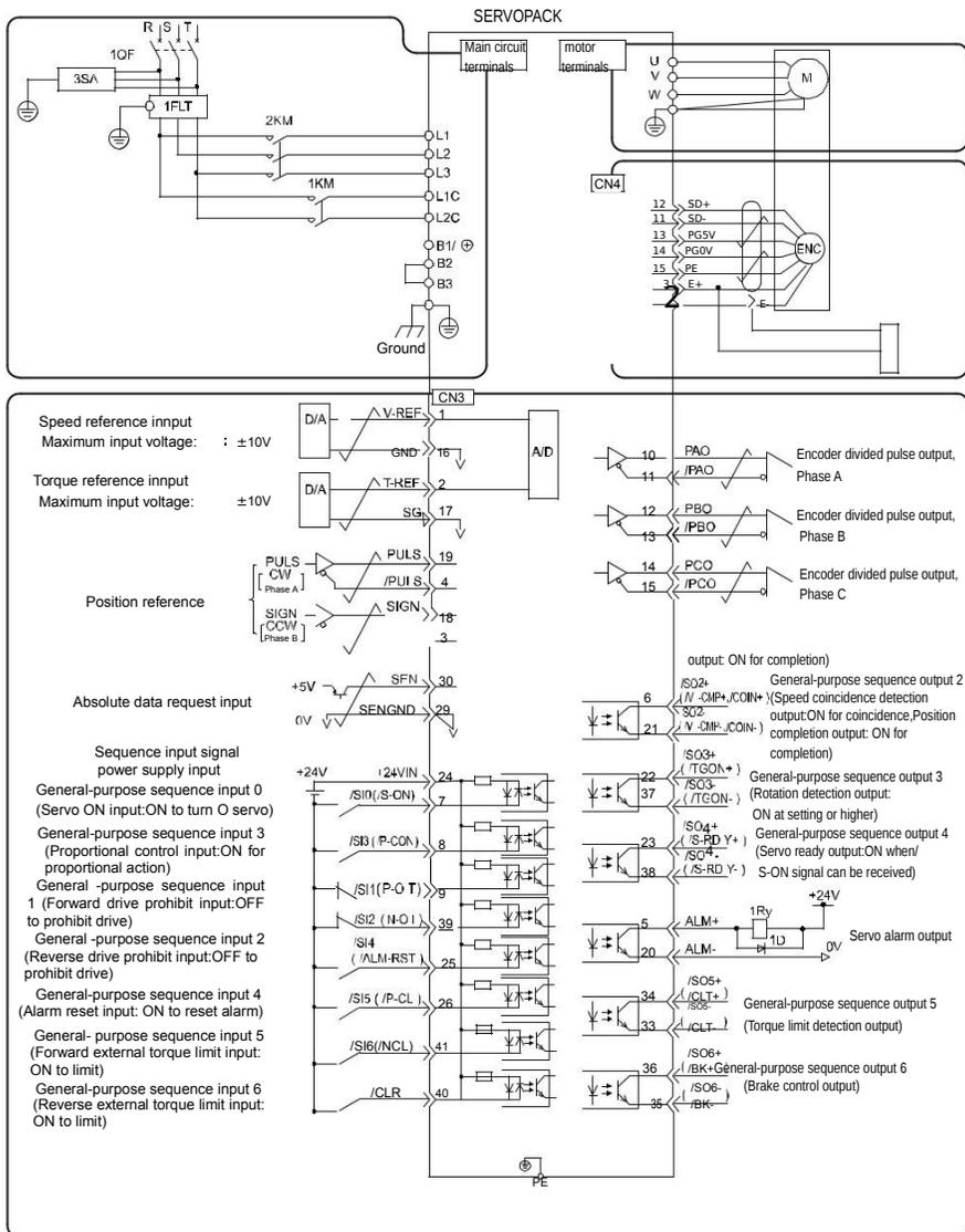
3.3 Wiring the Power Supply to the SERVOPACK
